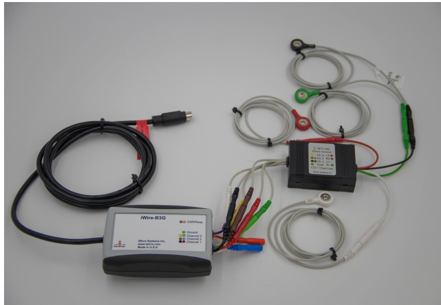
Figure HH-10-S2: iWire B3G connected to the Wilson Terminal.
